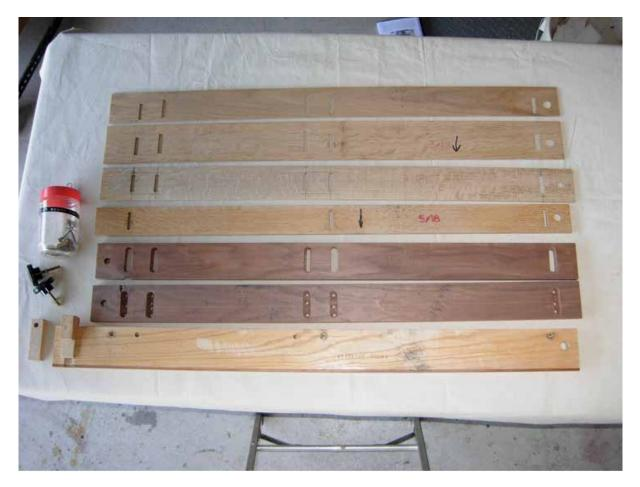
This is the set of Sticking boards and shims I made. The peanut butter jar holds the knobs and fasteners and has a hook to hang on the pegboard with the wooden parts.
