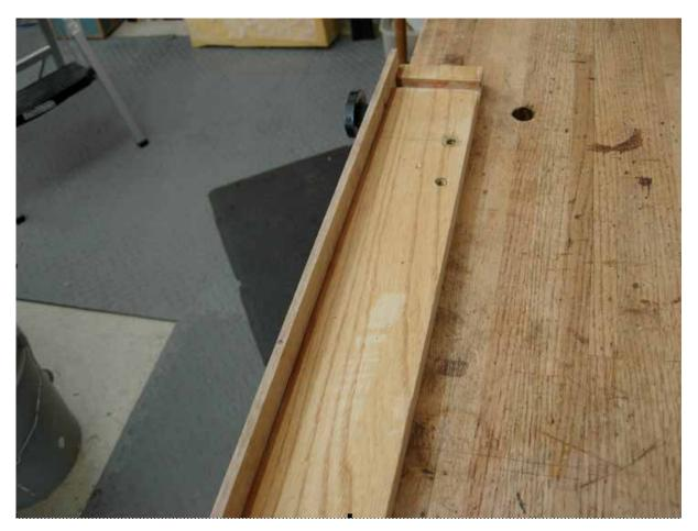
This is the view of the alignment fence installed from the back side. The next section will deal with the planes directly involved in shaping the sash components.
