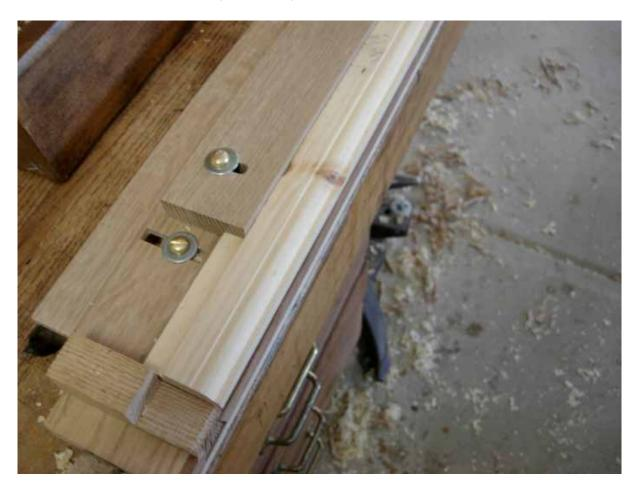
This shows the sticking board configuration when making the final cut to the molding.
