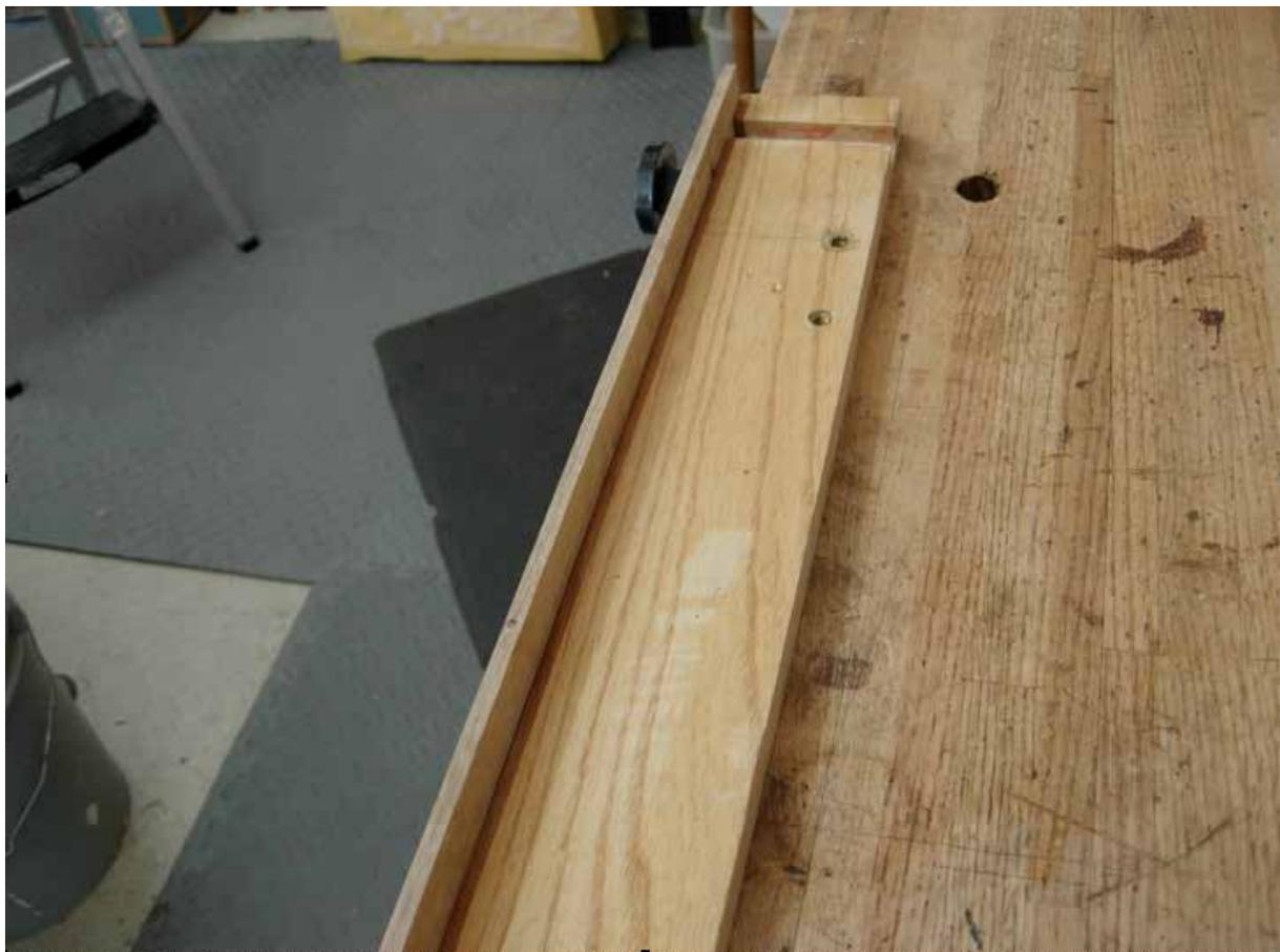
This is the view of the alignment fence installed from the back side.
