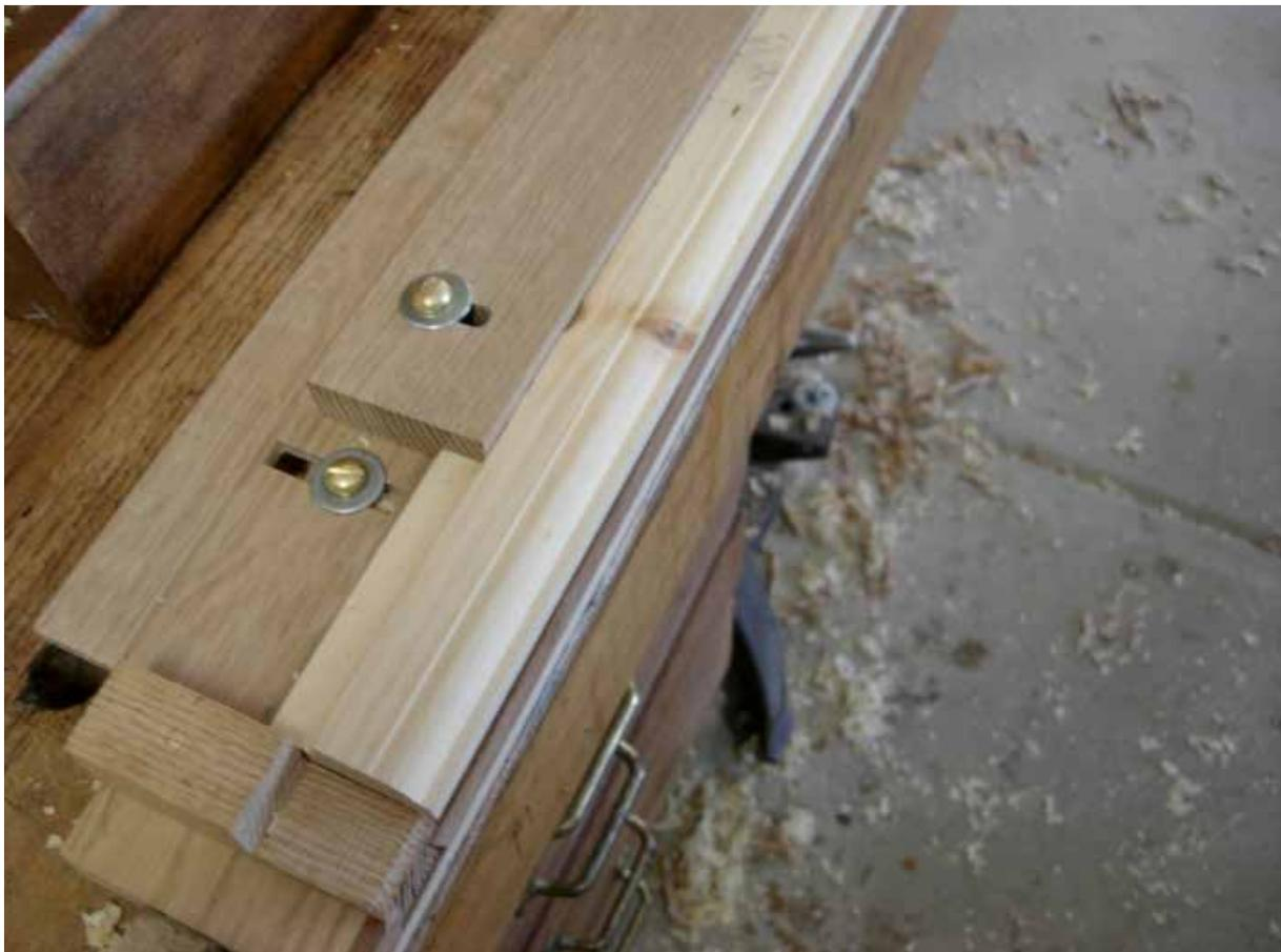
This shows the sticking board configuration when making the final cut to the molding.
